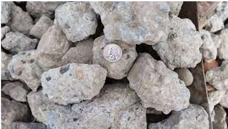
Picture 2. 2 Inch - 4 Inch Recycled Concrete 22
